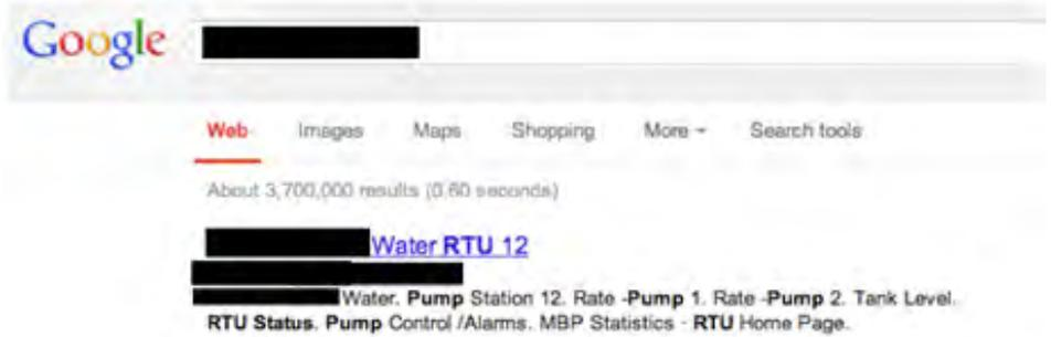
FIGURE 3: Google-dorks search that easily located a water-pumping station
