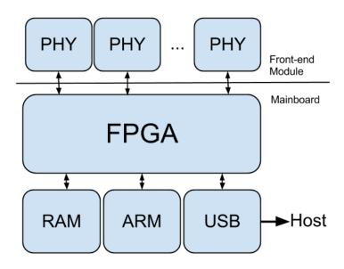
Figure 1: a high level view of the Daisho architecture
