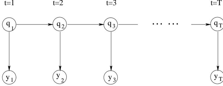
Figure 7: A representation of a trace of a HMM. Each vertical slice represents a time step. In each time slice, the top node  $q_t$  is a variable representing a character pair, and the bottom node  $y_t$  is the observable variable denoting the latency between the two keystrokes.
