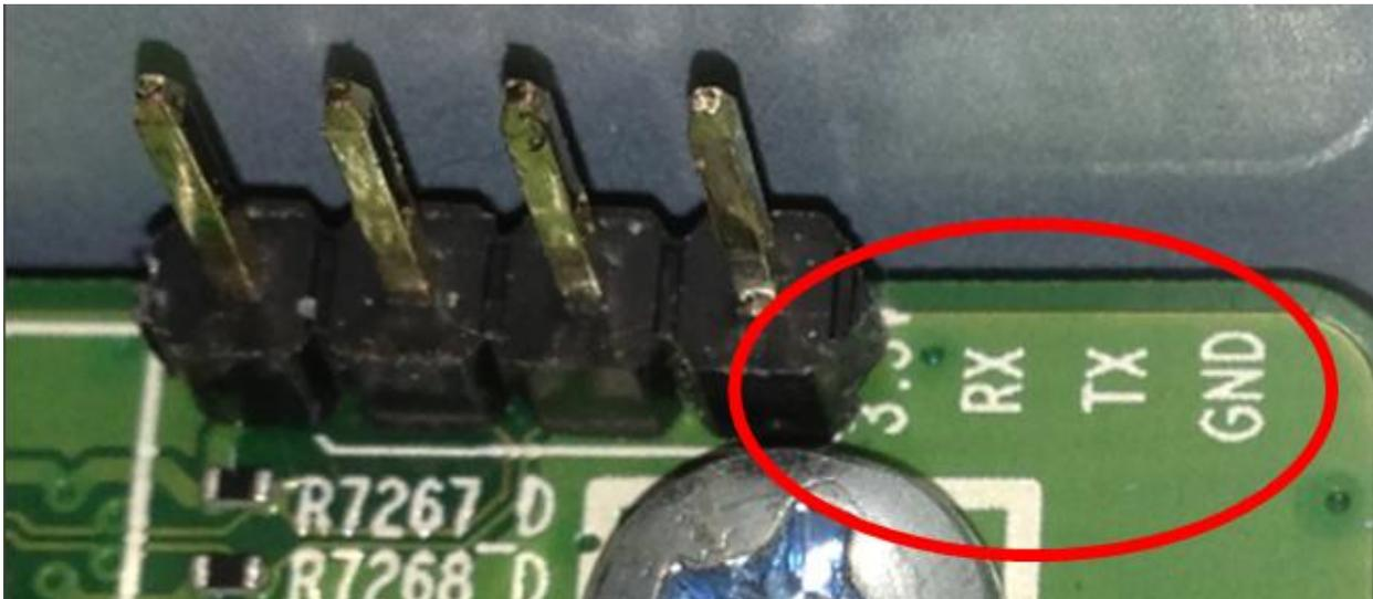
Figure 2 the four descriptions seen here are characteristic of UART
