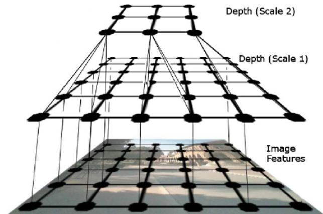
**Fig. 4** The multiscale MRF model for modeling relation between features and depths, relation between depths at same scale, and relation between depths at different scales. (Only 2 out of 3 scales, and a subset of the edges, are shown)
