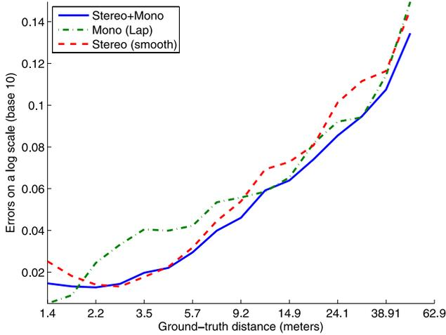
**Fig. 14** The average errors (on a log scale, base 10) as a function of the distance from the camera
