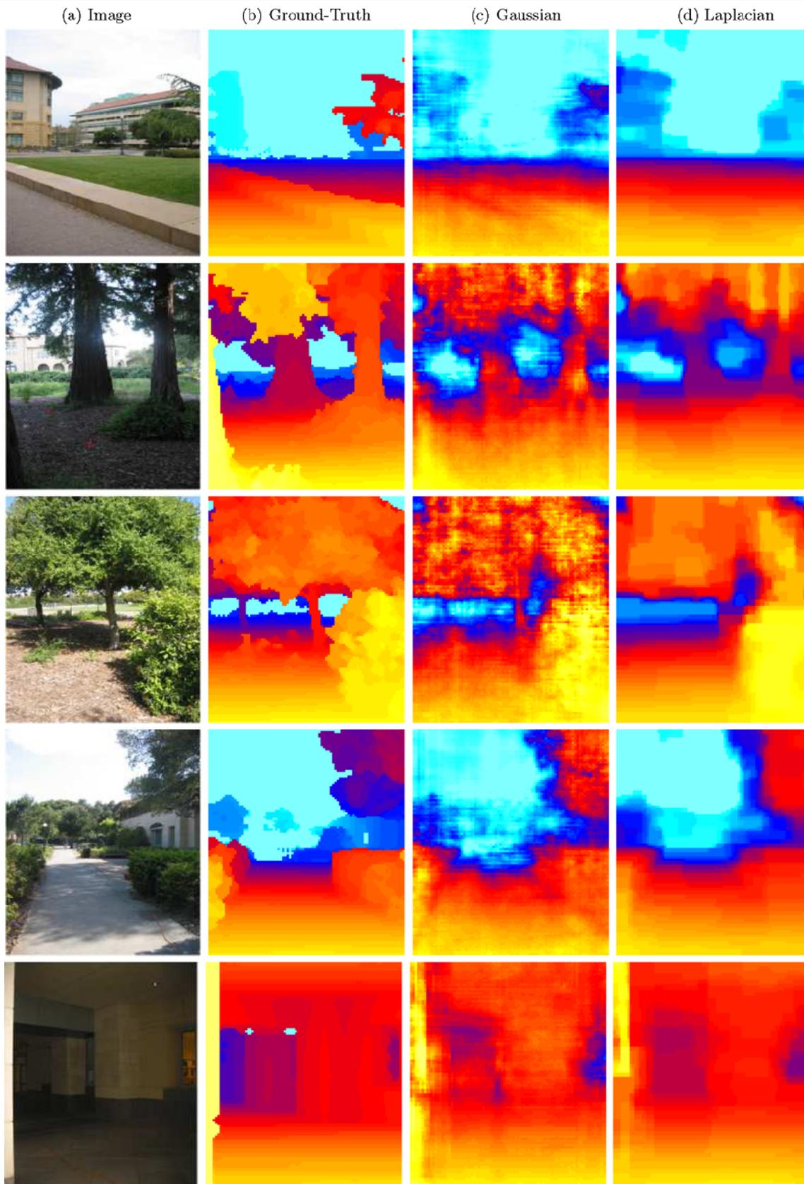
**Fig. 6** Results for a varied set of environments, showing **a** original image, **b** ground truth depthmap, **c** predicted depthmap by Gaussian model, **d** predicted depthmap by Laplacian model. (Best viewed in color)
