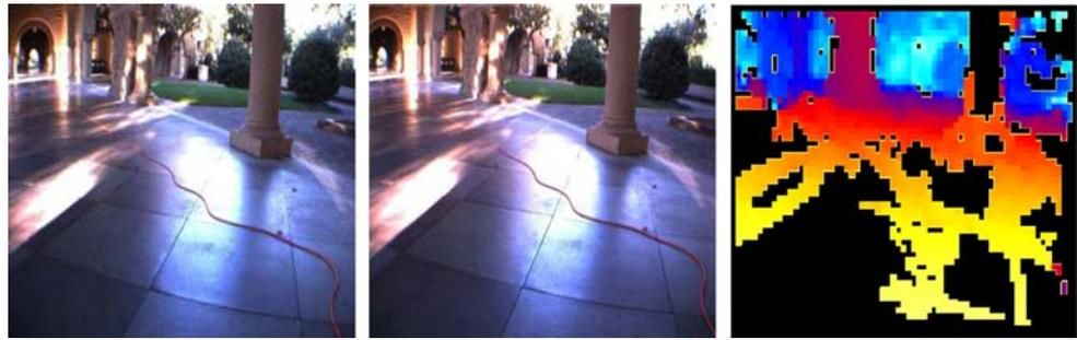
Stereo correspondences give reliable estimates of disparity, except when large portions of the image are featureless (i.e., correspondences cannot be found). Further, for a given baseline distance between cameras, the accuracy decreases as the depth values increase. In the limit of very distant objects, there is no observable disparity, and depth estimation generally fails. Empirically, depth estimates from stereo tend to become unreliable when the depth exceeds a certain distance.
