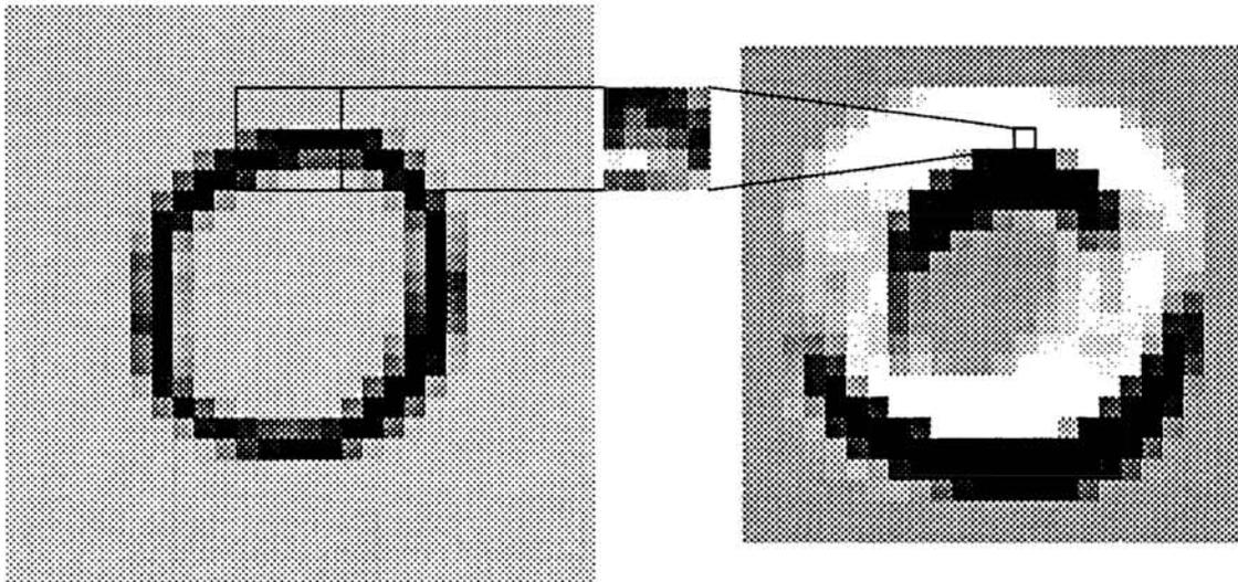
**Figure 3:** Input image (left), weight vector (center), and resulting feature map (right). The feature map is obtained by scanning the input image with a single neuron that has a local receptive field, as indicated. White represents  $-1$ , black represents  $+1$ .
