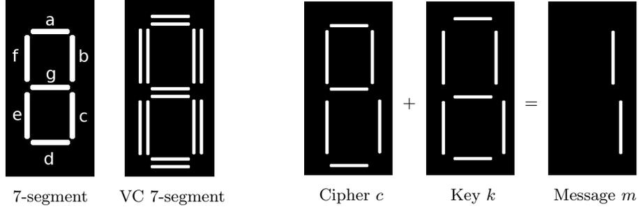
Fig. 2: Segment-Based Visual Cryptography on 7-segment Displays
