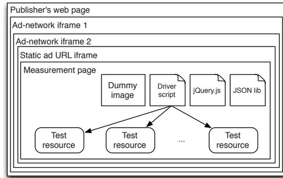
Figure 3: Client-side experiment setup
