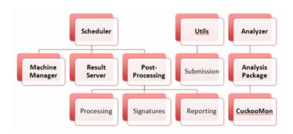
These phases of malware analysis can be customized almost completely. Machinery modules define how the virtualization solution is managed and VMs are started, restored and stopped.
